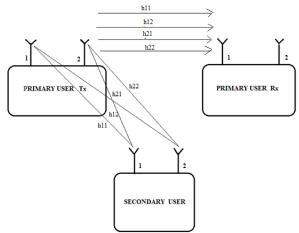
Fig 3. Basic Two –antenna MIMO System incorporated in CR.
